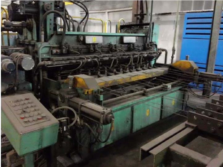
Wire Mesh Welder with Pneumatic Line Wire Advance System (Crank Drive) with Cutting Stroke
